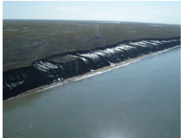
Figure 18. Northwest bank of Baillie Islands showing melting of ice-rich permafrost and bank slumping into the Beaufort Sea. Photo by Suzanne Carrière, ECC, 2011.
